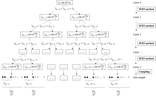
Figure 4. Flow chart of one generated l_k -out-of- m_k sample
