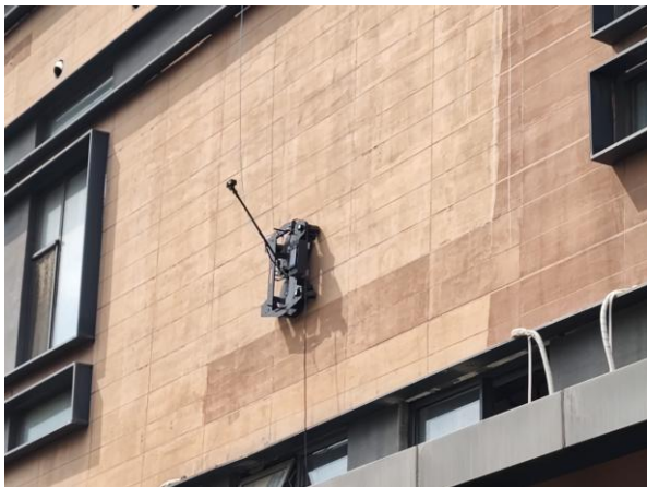
Figure 9. Building exterior inspection using the wall-climbing robot.
