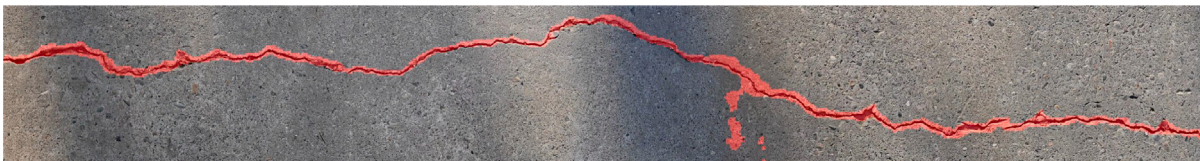
(e) DeepCrack detection, Sample 11
